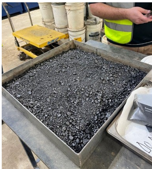
Figure 6: Graphite concentrate (93.4% graphite) sample used in purification tests 7
