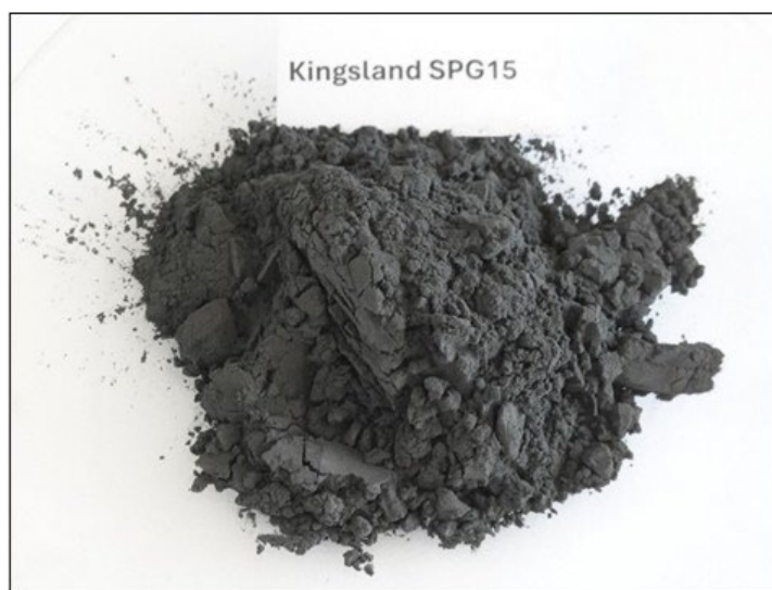
Figure 7: Sample of Spherical, Purified Graphite (PSG) >99.95% graphite, generated from Leliyn concentrate
