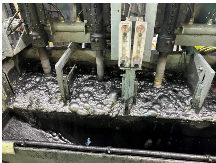
Figure 1: Flotation Cell producing graphite concentrate for bulk sample
