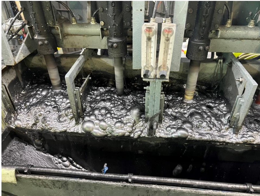
Figure 8: Flotation Cell producing graphite concentrate for bulk sample
