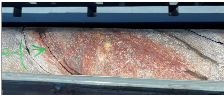
Figure 4: Drill Hole CLRC023 120.63m – 121.0m at 29,197ppm (2.91) U 3 O 8 6
