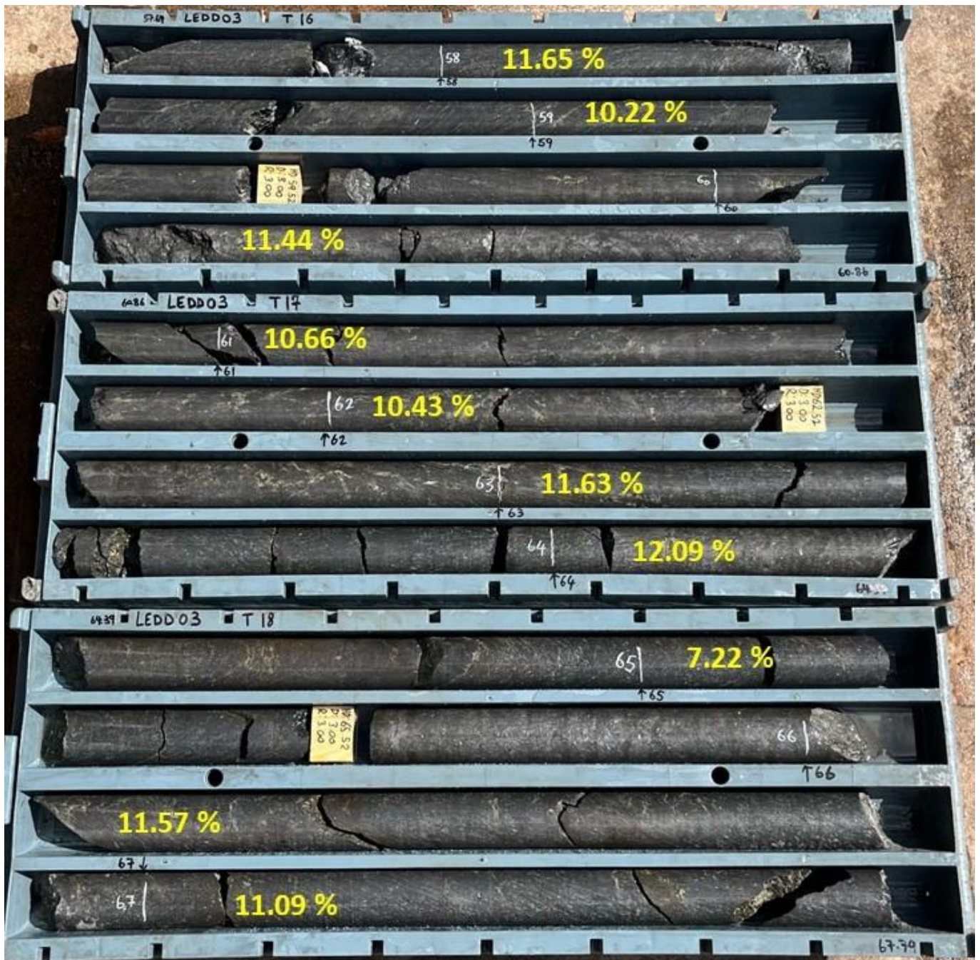
Figure 5: LEDD_03, 57m-67m showing 1 meter assay results
