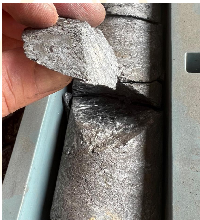
Figure 2: LEDD_03 18.5m 11.3% Total Graphitic Carbon
