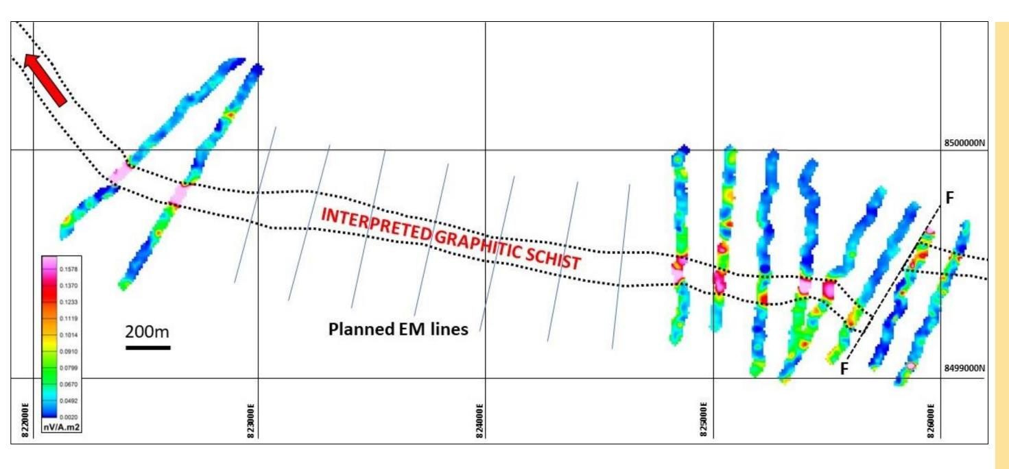
Ground EM survey successfully delineating graphitic schist within Exploration Target area.
